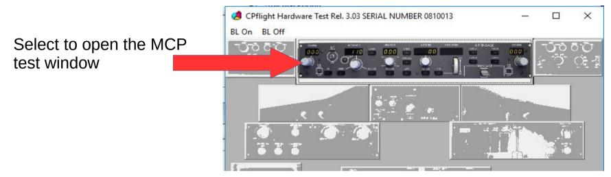
Test switches and Knobs. You will be able to see on the screen the hardware command
